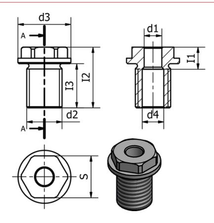
Tightening torque in Nm = 145
